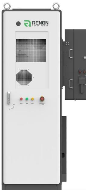
The ECube 60AP product has an energy capacity of 60kWh. Its main configuration includes: 12 set of battery packs, 1set of main control box, 1 set of 2kW air conditioner, and 1 set of fire protection system, 1 set of battery management system (BMS), and 1 set of communication management system.
